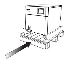
**Place** the front bar against the front of the pallet. Failure to complete this step can cause damage to the generator.
