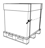
**Cut** the plastic strapping and **remove**.
