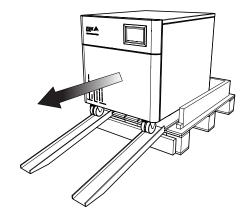
Release the brakes and carefully manoeuvre **Generator** down the ramps and into final position.
