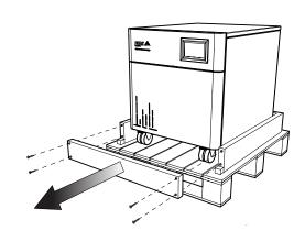
**Remove** the four screws shown, these will be marked in red and remove the front bar.
