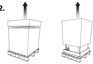
Remove cardboard lid, protective foam packaging and cardboard sleeve. Remove the plastic covering the generator.
