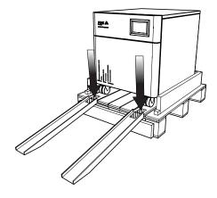
**Attach** the ramps to the front of the pallet using the hook and loop straps. Ensuring they are alligned with the wheels.
